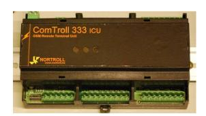
The ComTroll 333 ICU is especially suitable together with the ComTroll 115C QuickLink Collector. ComTroll 115C communicates with up to 9 LineTroll 110E $\mu$ R phase –mounted fault passage indicator with a 2.4GHz radio link.
