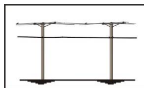
DISTRIBUTION SYSTEMS WITH EART-HWIRE
