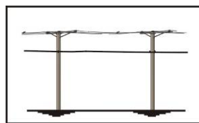
DISTRIBUTION SYSTEMS WITH EART-HWIRE
