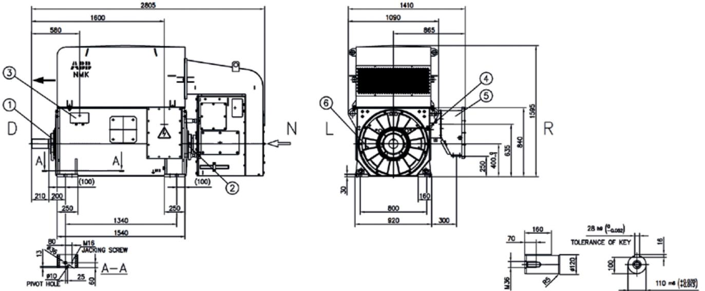
Antifriction bearings, IEC, 1 <math>U \le 6.6 \text{ kV}</math>, IM 1001, IC611 / IP55, >=4 pole, frame size 450
