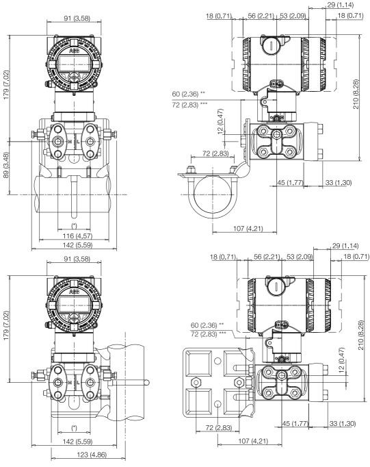
Fig. 7: Pipe mounting - Barrel housing
