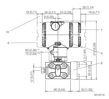
Fig. 5: Barrel housing - Horizontal flanges
