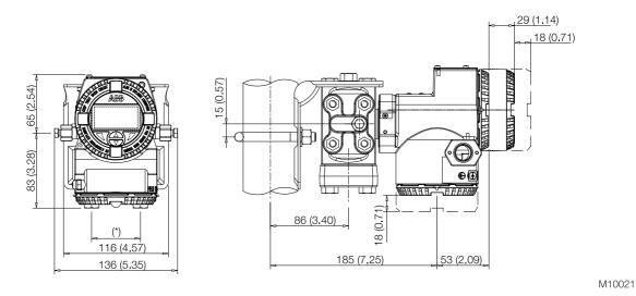
Fig. 8: Pipe mounting - DIN housing
