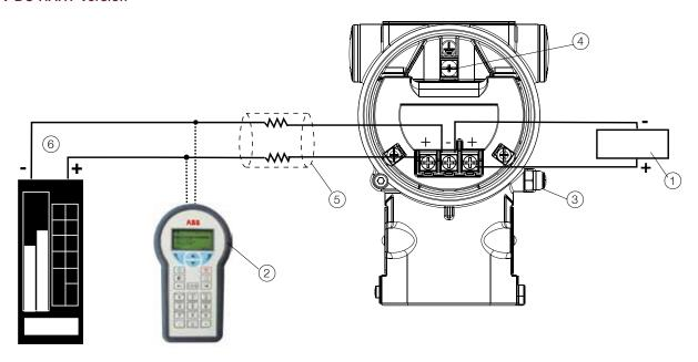
HART hand-held communicator may be connected at any wiring termination point in the loop, providing the minimum resistance is 250 ohm. If this is less than 250 ohm, additional resistance should be added to allow communications.
