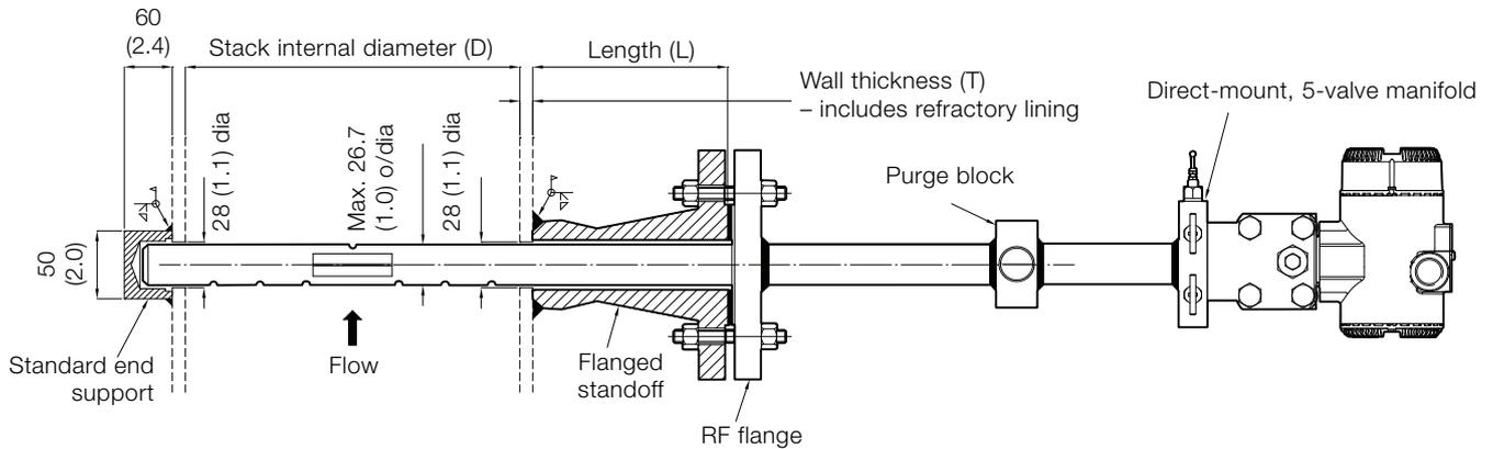
**Probe – 25 mm (1.0 in.) diameter with flanged end support (with integral transmitter)**
