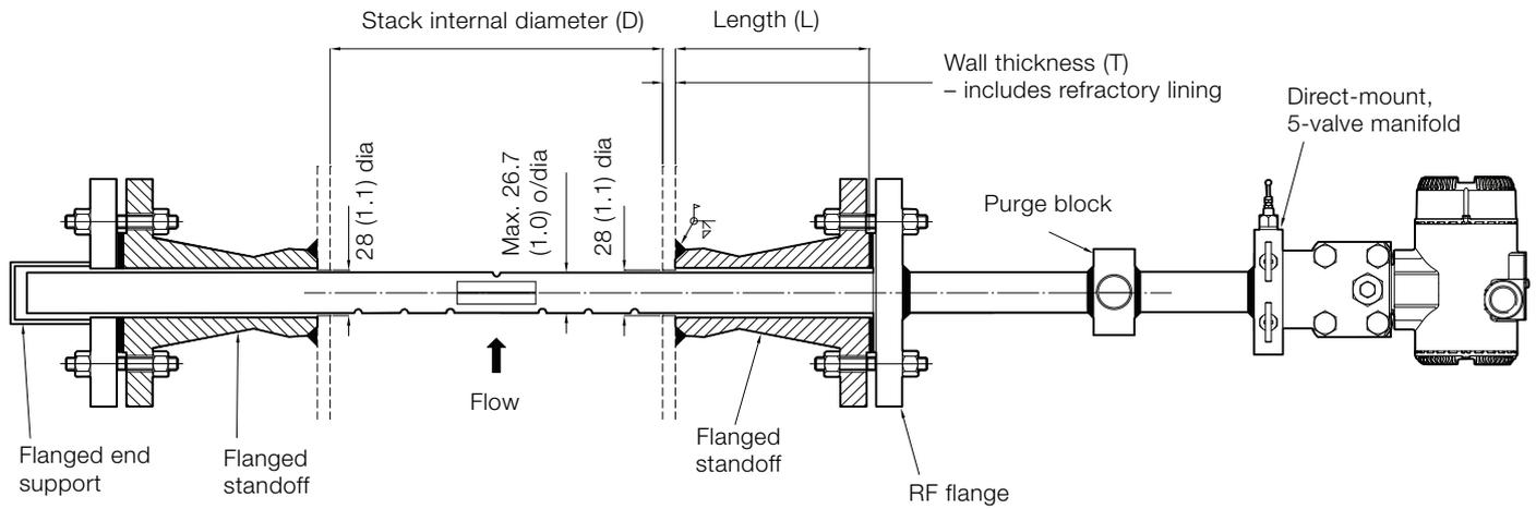
**Probe – 60 mm (2.4 in.) diameter with weldcup end support (for remote transmitter)**
